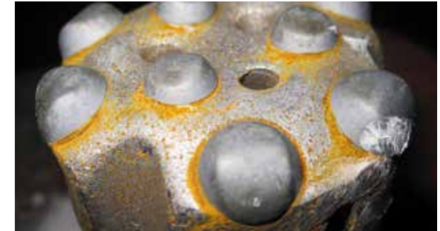
The height of the cemented carbide diminishes as wear progresses, resulting in a flat wear.
