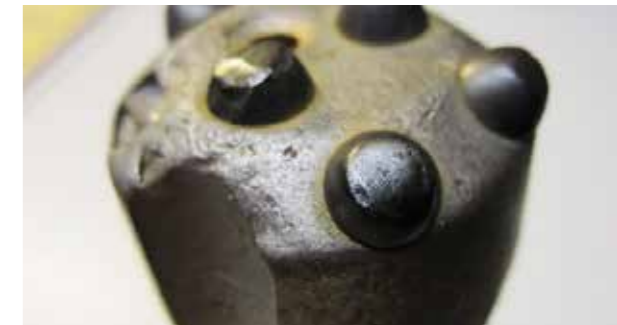
Wear to the cemented carbide on the periphery of the bit is abnormally high, causing an "anti-taper" to develop, which diminishes the clearance of the bit.
