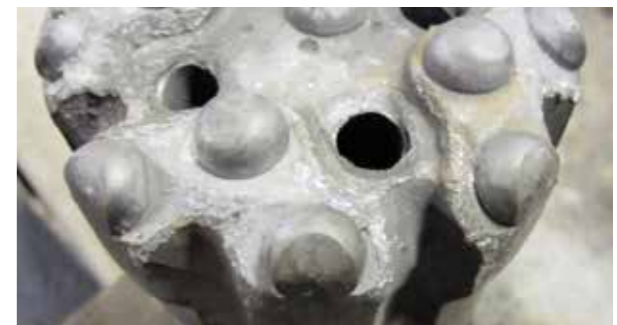
A fatigue surface with microscopic cracks (snakeskin).
