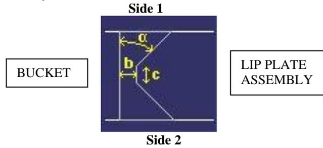
Fig. 1. Double-bevel butt weld preparation
