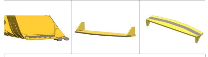
5. To weld the parts to the bucket or lip follow the relevant OEM welding procedure (options shown below):
