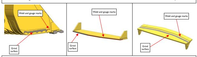
4. Perform NDT (Non-Destructive Testing) on the gouged area of the bucket to ensure no cracking exists. If cracks are found regrind to remove entire cracks and rewell according to PWP0001 and relevant OEM welding procedure:
