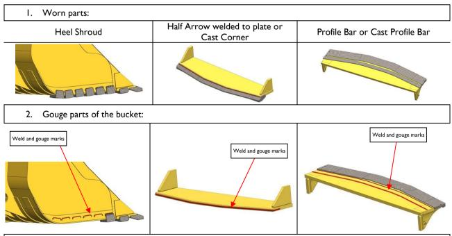
When removing Heel Shrouds, Half Arrow and Profile Bar ensure OEM manufacturing procedures, local site safety procedures, and welding procedures are followed.
