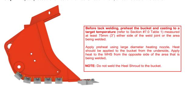
**Step 5**: If temperature is below minimum preheat temperature, reheat the weld area to the target preheat temperature.
