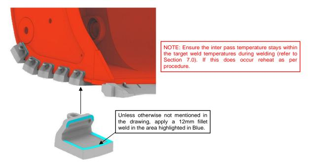
Step 7: Fill out weld prep on both side of the bucket with as many runs as required.
