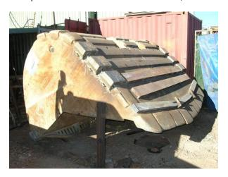
Step 2: Mark placement of new heel shrouds.
