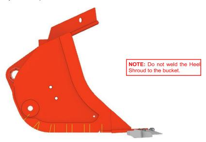
Step 3: Lift Heel Shroud in place and tack weld onto the bucket (ensure safe lifting).
