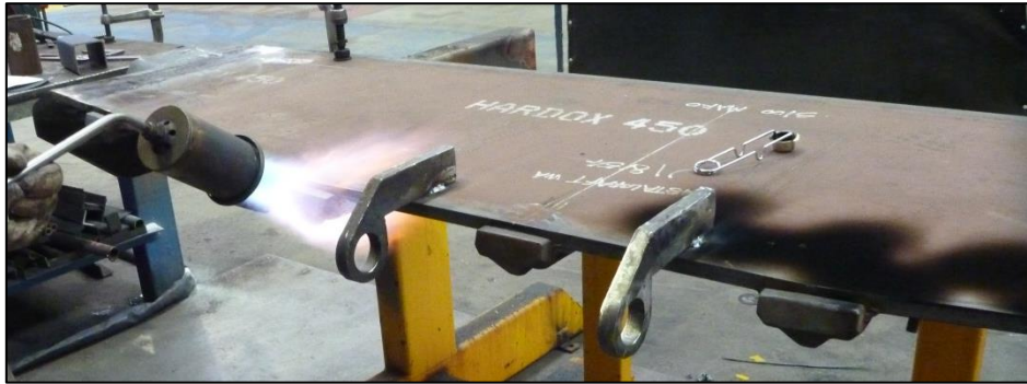
Figure 31 Pre-heating at 1G position
