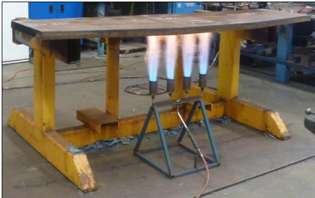
Figure 3 Preheating Hardox plate
