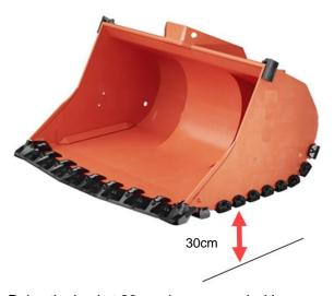
Raise the bucket 30cm above ground with proper support.
