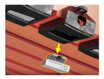
Push the nut away from you and remove the nut from the heel shroud cavity.
